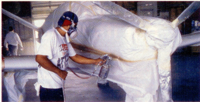
Heriberto Diaz masks striping on the Bonanza's wing tip (far left). Murmer's Lupe Lopez Jr. sprays gold trim over the white base coat (left).
