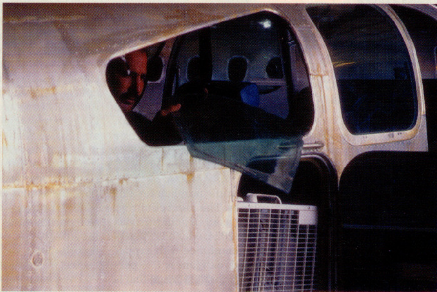
Stripped and masked for painting, the AOPA Sweepstakes Bonanza sits in front of Murmer Aircraft Services in Arcola, Texas (above). A fan keeps Doug Kelly cool while he's installing the new Beryl D'Shannon windows (left).
