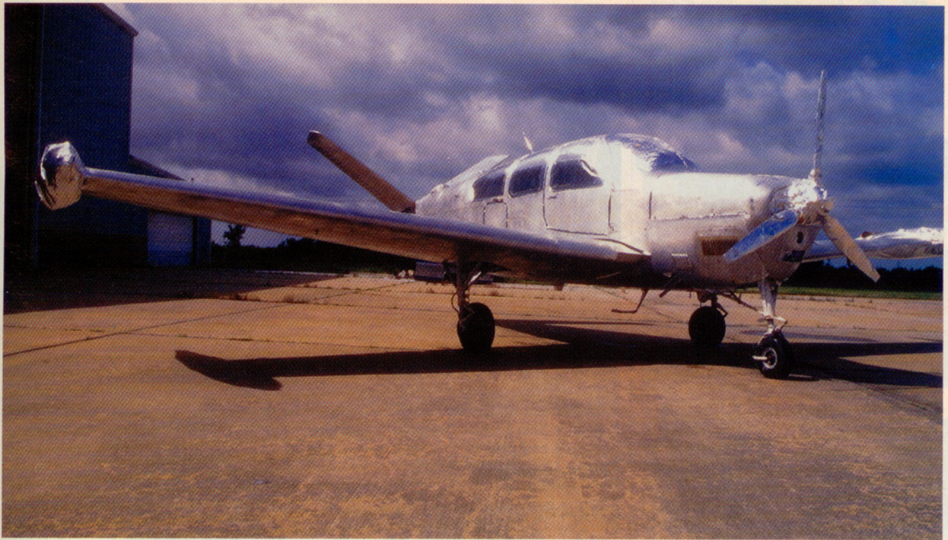
Stripped and masked for painting, the AOPA Sweepstakes Bonanza sits in front of Murmer Aircraft Services in Arcola, Texas (above). A fan keeps Doug Kelly cool while he's installing the new Beryl D'Shannon windows (left).
